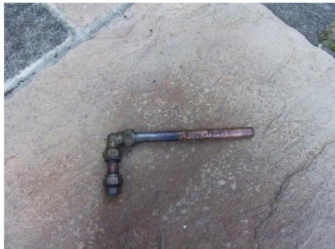
The vaporiser is made up of 2 sections of either 15mm or 20mm copper pipe, with one horizontal 200mm long section and the 2<sup>nd</sup> vertical 50mm section. Sizes are only a guide and are not critical. The bend is a right angle brass compression fitting.
